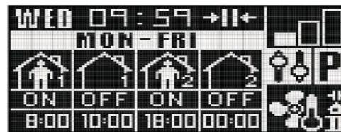
An example of the programmed calendar (working days). The device will be switched on at 8 a.m. and it will be switched off at 10 a.m. It will be switched on again at 6 p.m. and it will be switched off at 12 a.m. The cycle shall be repeated from Monday to Friday.
